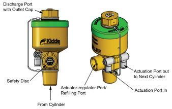
Figure 4. Valve Components The Natura IGS valve assembly has a 3/4 in. (20mm) discharge port with BSP male threads.
