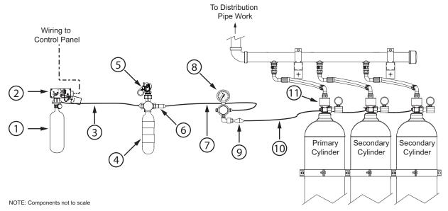
Figure 3. System with Discharge Delay
