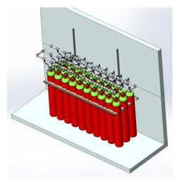
Figure 16. 80L Cylinder Racking Example
